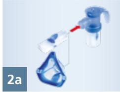
**2a** Attach the mouthpiece or the mask to the nebuliser.
