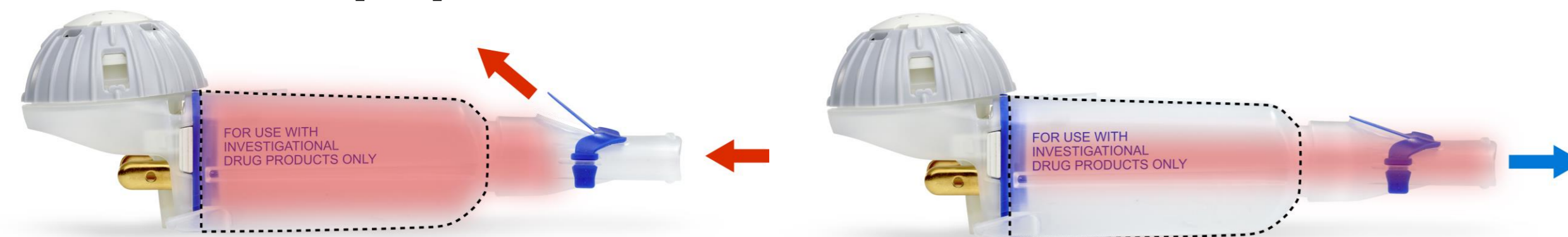
Figure 1: Investigational PARI eFlow nebulizer during exhalation (left) and inhalation (right)
