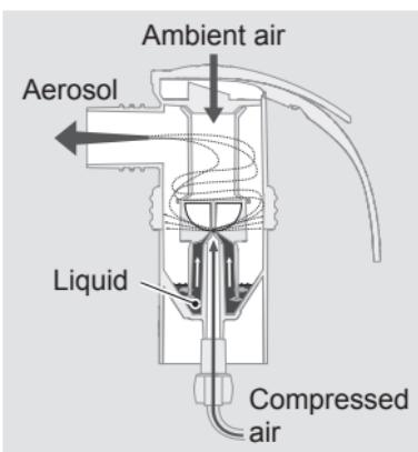
The size of the aerosol droplets is determined by the nozzle inserts. The smaller the droplets are, the farther they can penetrate into the deeper and smaller regions of the lung:
