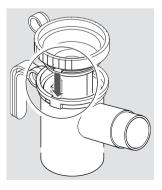
• Attach the connection tubing to the nebuliser.
