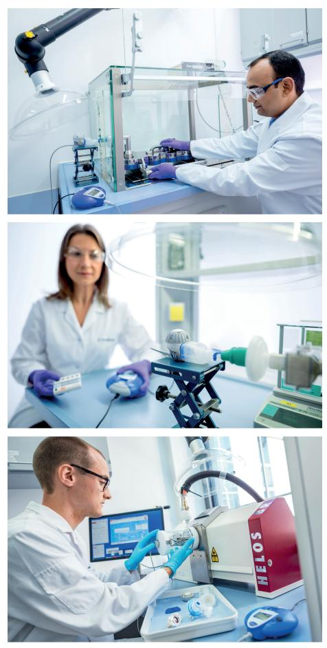
Figure 3: During the feasibility phase – (top to bottom) NGI, breath simulator, and laser diffraction measurements.
