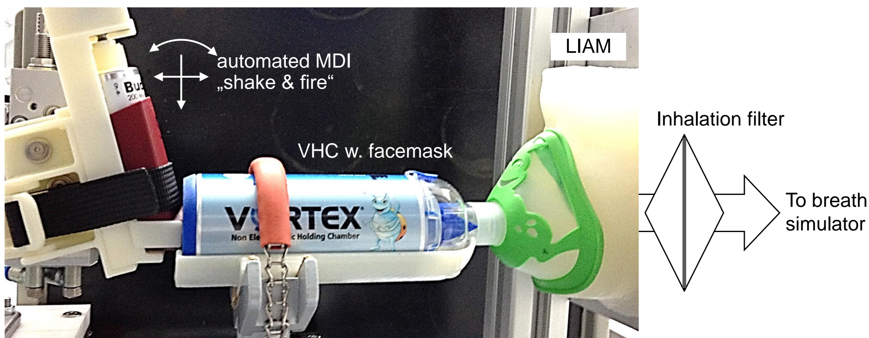
Figure 2: Breath simulation experiment with face model LIAM, VHC with facemask and automated MDI shake and fire system for synchronized time delay simulation.
